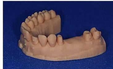
1. figure: 3D printed, solid dental model
